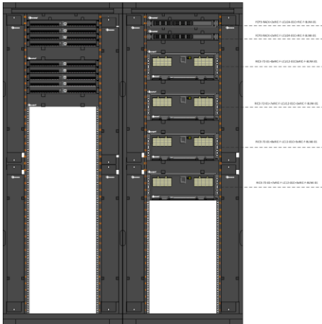
Typical view for CPZ cabinets located in MDA ZONE/TELECOM AREA (one cabinet for fibre connections and other for copper connections)
