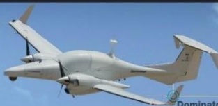
Dominator UAV Aeronautics Operational Altitude: 30,000 feet Wingspan: 13.5m Endurance: 28h
