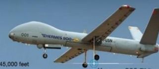
Hermes 900 Elbit Operational Altitude: 33,000 feet Wingspan: 15m Max Payload Weight: 300Kg Endurance: 40h
