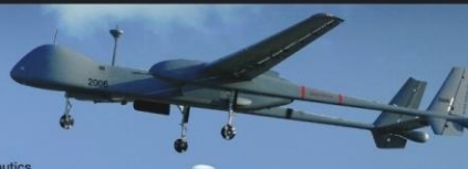
Heron TP IAI Operational Altitude: 45,000 feet Wingspan: 26m Max Payload Weight: 1000+Kg Endurance: 36h
