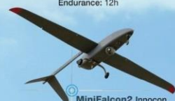
MiniFalcon2 Innocon Operational Altitude: 18,000 feet MTOW: 150kg Wingspan: 5.5 meter Endurance: <15 hours Max. Payload weight: <35kg
